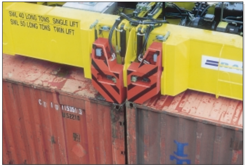
Figure 4 (top) Twin-20 detection system mounted on the underside of a Bromma twin-lift spreader at the Port of Miami
