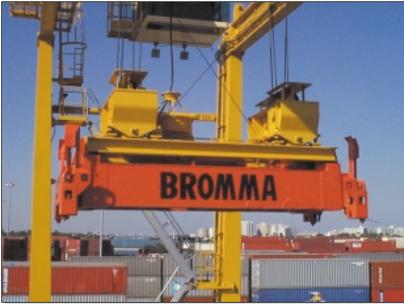
Figure 6 Specially designed Interface Frame on new Mi-Jack RTG for the Port of Miami Container Terminal
